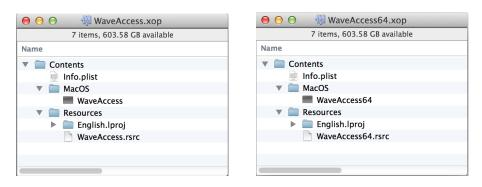
In order for the XOP to load, the package name (e.g., **WaveAccess**.xop) must agree with the executable name (e.g., Contents/MacOS/**WaveAccess**) which must agree with the value of the CFBundleExecutable key in the Info.plist file (Contents/Info.plist). If any of these names are incorrect, Igor will be unable to load the XOP and usually will report "Can't load the executable file in the XOP package".
