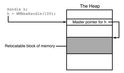
Igor uses Handles mostly for passing variable-length data, typically strings, to an XOP, and for receiving variable-length data from it. You use routines described under **WM Memory XOPSupport Routines** on page 195 to deal with Handles.
