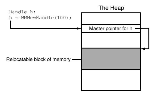
Because a handle refers to a block of memory indirectly, you must "dereference" the handle before you can access the block. For example, if h is a handle returned by WMNewHandle, then \*h is a pointer to the block of memory that h refers to.
