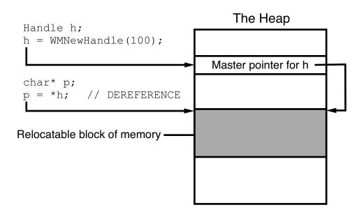
The pointer p now points to the block in memory and we can access the data using it.
