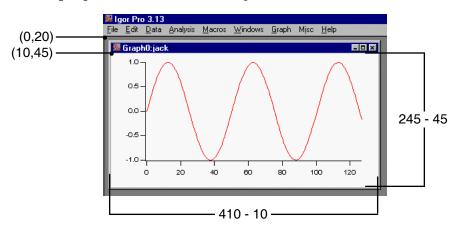
On Windows the correspondence between points and pixels is set by the Display control panel. Igor coordinates are stored as floating point because, to accurately reposition a window, we need to use fractional points in /W=(left,top,right,bottom) flags.
