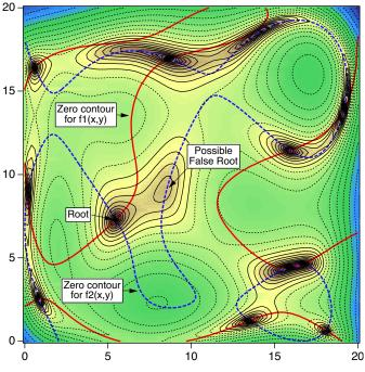
The thin lines are contours of  $f1(x,y)^2+f2(x,y)^2$ , with dotted lines for high values; minima are surrounded by thin, solid contours. You can see that every intersection between the heavy zero contours is surrounded by thin contours showing that these are minima in the sum of the squared functions. One such point is labeled "Root".
