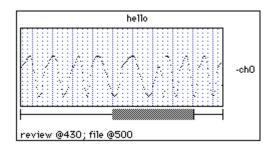
Notice the positioning strip just under the chart and above the status line. It consists of a horizontal line and a horizontal, gray bar. The line, called the positioning line, represents the extent of available data. The bar, called the positioning bar, represents the currently displayed region of this data.
