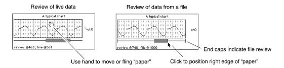
While data acquisition is in progress, the horizontal line represents the extent of the data in the FIFO's memory. After acquisition is over then the line includes all of the data in the FIFO's output file, if any.
