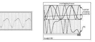
A given chart recorder control can monitor an arbitrary selection of channels from a single FIFO. Each trace can have its own display gain, color and line style and can either have its own area on the "paper" or can share an area with one or more other traces. There can be multiple chart recorder controls active an one time in one or more panel or graph windows.
