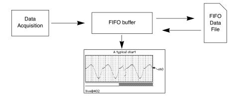
A FIFO can have an arbitrary number of channels each with its own number type, scaling, and units. All channels of a given FIFO share a common "timebase".
